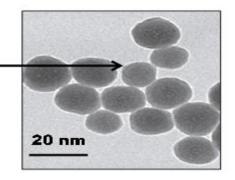
Fig. 3. Transmission electron micrograph of biostabilized PdNPs
